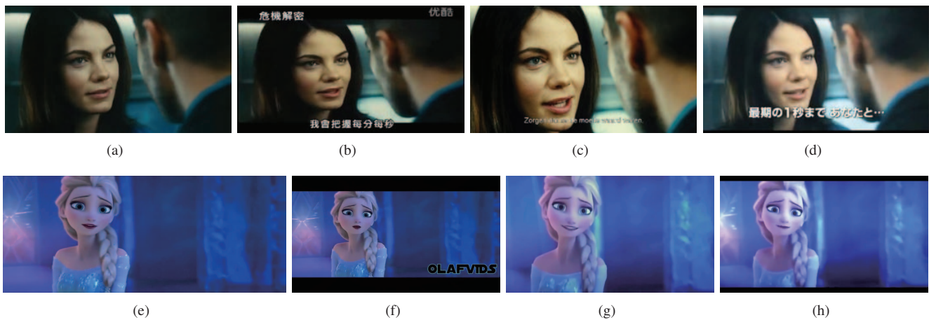
Fig. 3. Examples of NDV detection results. The videos in the same row are clustered into the same near-duplicate group by the proposed algorithm. Original contents in (a) and (e) are edited with various near-duplication types, such as logos and subtitles (b, c, d, f), cropping (c, g), and photometric variations (b, c, d, g, h).
